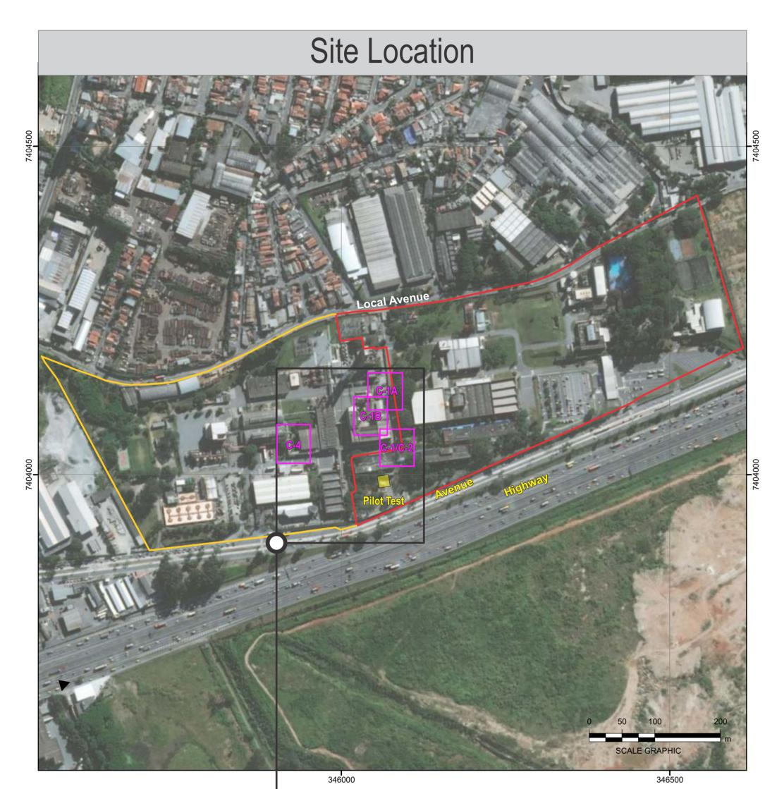
Following the pilot test, the first stage of the full scale remediation was performed in May 2019, and the second stage between November 2020 and February 2021.
